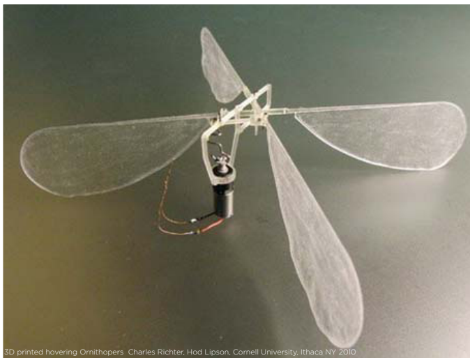
3D printed hovering Ornithopters. Charles Richter, Hod Lipson, Cornell University, Ithaca NY 2010.
